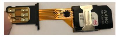
**3.** Fold the ribbon around the left side of the simtray, and fold it to the back.
