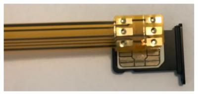
**2**. Put the SIM card in the simtray. Then place the adapter on the SIMcard as shown in the picture.
